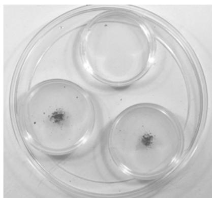
**Fig. 1.** Klason lignin degradation test: *Fusarium solani* f. sp. *glycines* as mycelial plugs was placed on a layer of Klason lignin in two petri dishes, while a third dish contained 20% KOH in order to trap the <sup>14</sup>CO<sub>2</sub> produced as a result of lignin degradation. The large petri dish was 15 cm in diameter and the small ones were 6 cm in diameter.
