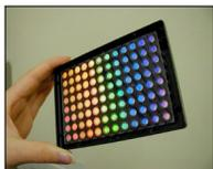
Photonic crystal biosensor embedded into the bottom of a 96-well microplate
