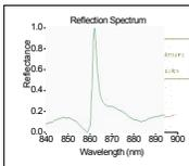
Reflectance before and after attachment of biomolecules
