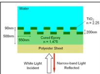
Cross section of the photonic crystal biosensor structure
