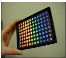
Fig. 2. Photonic crystal biosensor embedded into the bottom of a 96-well microplate [3]
